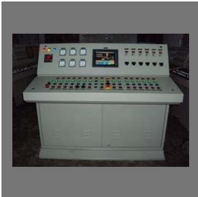
Wet Mix Plant Control Panel
