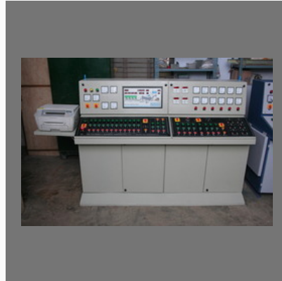
Asphalt Drum Mix Plant Panel
